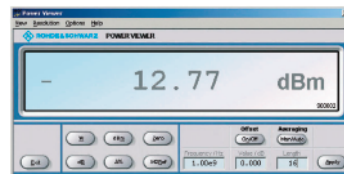
The Power Viewer turns any PC into a power meter
